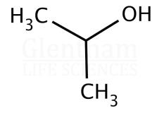
PropertySpecificationPhysical DescriptionClear, colourless liquidWater $\leq 0.005\%$ Residue on Ignition $\leq 0.0005\%$ Assay $\geq 99.9\%$
