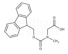
PropertySpecificationPhysical DescriptionWhite to almost white powderSolubility (5% in DMF)Clear, colourless to very faint yellow solutionMelting Point110.0 - 120.0 °CWater (KF)≤ 6.0%Assay (Titration)≥ 98.0%
